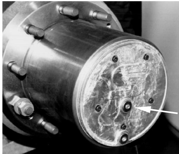
**Picture 18. Oil level plug in the planetary wheel hub.**
