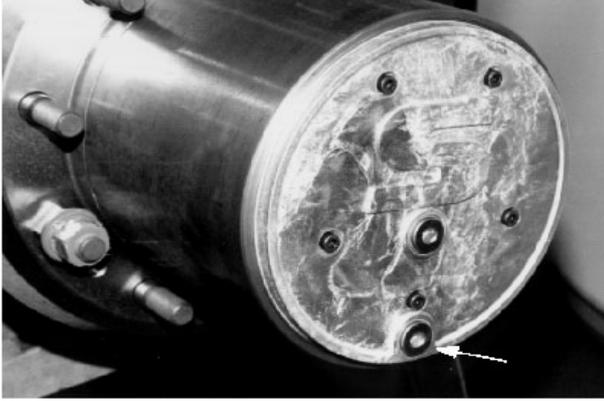
**Picture 1. Wheel hub drain plug**
